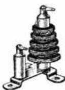
Isolantite mounted choke for medium and high power transmitters. Two types, one for 160 and one for 40 meters. Insulated for 10,000 volts. Inductance 4 millihenries; distributed cap., 1
