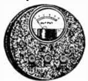
A practical instrument for measuring output of a radio net when used in conjunction with an oscillator for aligning R.F. and I.F. circuits. Contains copper oxide rectifier. Two ranges available: 0-5 volts for connection to voice coil, 0-50 volts for connection to plate of tube. Model 555 mounted on metal panel with jacks and test leads. Shpg. wt. 4 lbs.
