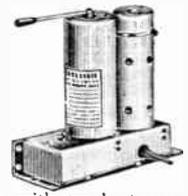
For use with any short wave superhet having intermediate frequency between 415 and 700 K.C. Receiver must also be able to supply power for additional tube filament. Just three wires to connect. For 2.5 volt sets, use 58 tube; a 6D6 with 6.3 volt sets. Unit is of the electron coupled type. Control rod varies pitch of note. Entire assembly on metal chassis 7x2¾x7". Shpg. wt. 7 lbs.
