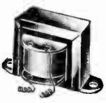
For coupling a screen grid tube to an audio stage. Will provide approximately 3 times the gain of resistance coupling. Inductance 1080 henries at 8 M.A. maximum D.C. Has leads. Size: 1 3/4 x 2 1/4 x 2" high. Shpg. wt. 3 lbs. **YE5497—Screen Grid Coupler Your Cost . . . \$1.73**
