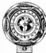
Improved type. Affords a ratio of 6 to 1 in 180°. Two scales on a translucent dial; upper scale calibrated from 0 to 100 and lower scale from 100 to 0. Knife edge pointer covers entire scale. Diameter of scale 3½". Comes with escutcheon plate. Shpg. wt. 1 lb.
