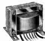
Open type with long coded leads. Have primary, high voltage and rectifier filament windings. Deliver full rated voltages and current. Primaries for 105-120 volts, 50-60 cycles A.C. Average size  $3 \times 2\frac{1}{2} \times 2\frac{1}{2}$ ". Shpg. wt. 4 lbs.
