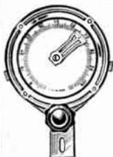
A new 3" dial designed for use with short-wave receivers, laboratory instruments, etc. Dial can be accurately read to .1 of one division. Open vision pointer permits addition of other bands in the center of the scale. Provides a spread of 270° for 180° condenser rotation. Dial ratio 14½:1, free from backlash. Plated scale and
