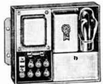
Delivers A.C. from a 6 volt battery. Taps at 90, 135, 180 and 250 volts. Battery drain only 4.0 amperes. Uses type 84 rectifier. Shpg. wt. 15 lbs.
