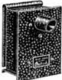
When used in conjunction with suitable "Light Source," the "Eye" may be used as counter, sorter, checker, in alarm systems, window displays, and for many other industrial and experimental applications. Consists of caesium cell, relay with heavy contacts, and amplifying stage. Shpg. wt. 6 lbs.
