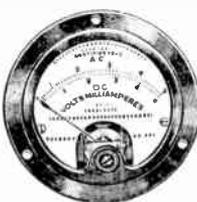
Designed for use with external resistances and shunts for measuring D.C. voltages and current and A.C. voltages. Of the permanent magnet moving coil type with a self-contained copper oxide rectifier for A.C. measurements. Self-contained for 5 volts and 1 mill. A.C., and 50 millivolts and 1 mill. D.C. Accurate to within 2% D.C.—5% A.C. YJ10774—List \$19.00
