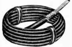
40 strands No. 29; 14-gauge. Layer of heavy cotton under covering of live rubber. Tinned. Ideal for heavy duty filament in transmitting apparatus. Shpg. wt. 25 ft., 1 lb.
