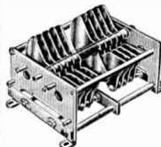
A new line of improved transmitting condensers designed for maximum obtainable efficiency. The frames are extremely rigid and are arranged for mounting on panel, chassis or stand-offs. The plates are of heavy aluminum with rounded and buffed edges. Front bearing is conical, rear bearing radial with single-ball thrust. Insulation is Isolantite, located outside of the concentrated field. Heavy duty construction with high peak voltage rating make them particularly attractive for use by the "Ham."
