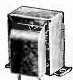
Fully cased filter choke rated 8.75 henries, 130 M.A. (inductance measured under full load). Has D.C. resistance of 231 ohms. 1600 volt insulation. Size: 3 1/2 x 2 1/4 x 3"; mtg. centers 3 3/8". Shpg. wt. 4 lbs. List price \$3.25. **YA269—Your Cost . . . \$1.90**
