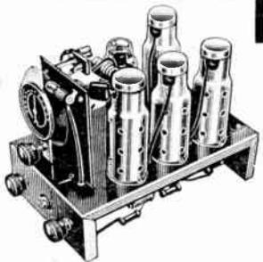
A hi-gain high efficiency ultra high frequency 5 tube receiver for the ham or short-wave enthusiast. Gives real super-heterodyne performance yet lacks the "hiss" so objectionable in this type of set. Bands covered 2 1/2, 5 and 10 meters using plug-in coils supplied with receiver. Either 6.3 or 2.5 volt tubes may be used, and the following are the types employed:
