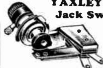
Jack Switch lies parallel with panel. Furnished complete with Black Knob; on-off plate. Mounts in 1/4" panel hole, up to 1/4" thick. Is 1 1/4" deep.
