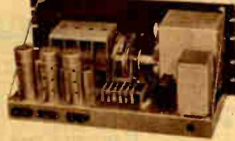
No longer is it necessary to be at the P.A. rack to tune the radio tuner from station to station or to control the volume. All tuner operations - tuning - volume adjustment - turning it on or off - can be done at a remote point, quickly, at the touch of a fingertip, with this new Lafayette Remote Control Tuner.
