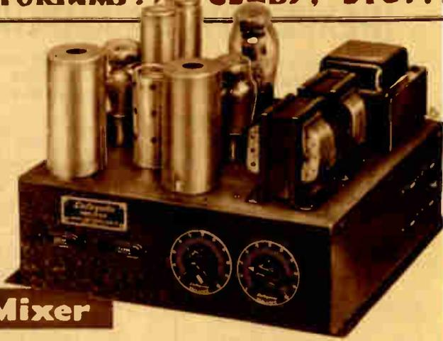
ONE of the most efficient amplifiers ever developed - has sufficient gain to use high impedance velocity microphones and crystal microphones without additional pre-amplification. Has a gain of 112 db, yet uses only a total of six tubes. Two 6C6's are used as electronic mixers, 79 as phase inverter and two 6B5's in the output stage. A 5Z3 tube is used as rectifier.
