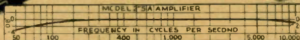
Curve given below shows the unusually flat frequency response characteristics of the 254-A amplifier.
