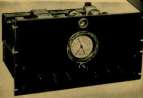
Illustration at left (above) shows neat panel arrangement. Tuning eye above the dial.
