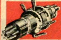
Covers frequency range of 2650 to 3330 mc/sec. Can take up to 75 watts input with forced air cooling. Frequency adjustable by means of screw (coarse) and knob (fine). Ratings: Beam V = 1000 at 40 ma, R.F. Power = 400. Filament is 6.3 v, at 3 amp. Reflector voltage—250.
