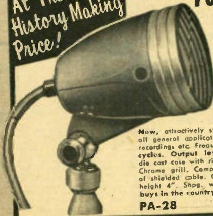
Now, attractively styled crystal microphone for all general applications—public address, home recordings etc. Frequency response 30 to 10,000 cycles. Output level—52 db; tilting head, die cast case with rich gray baked enamel finish. Chrome grill. Completely equipped with 5 feet of shielded cable. Grill dia.  $2\frac{1}{4}$ ", depth  $3\frac{3}{4}$ ", height 4". Shpg. wt. 3 lbs. One of the best buys in the country.
