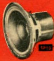
Model SP8B Radax Super-Eight. 8-inch coaxial speaker. Resonance 65 cps. 15-20 watts. Response 35-13,000 cps ± 6 db. 16 ohms impedance. Sens. rig. 44 db. Crossover, 6000 cps. 1 lb. Alnico V magnet. 8 1/2" diam., 7" baffle opening. 4 1/2" depth behind mtg. panel. Shpg. wt. 8 1/2 lbs.
