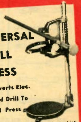
Here is a handy accessory item which acts as a drill stand and converts any 1/4" electric hand-drill into a drill press. Maximum length of travel is 2 1/2". Overall height is 14 1/2". Sturdily constructed. Powerful spring holds drill in place when not in use. Shpg. Wt. 9 lbs.
