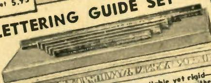
Made of transparent plastic that's pliable yet rigid—a must for good lettering. Simple to use with either sharp pencil or ink. Each guide has undercut to prevent ink smears when moved. Each has complete alphabet, all numbers plus commonly used signs. Most letters formed with one operation. Set consists of 1/2" guides. Sizes 1/4", 3/16", 1/4", 5/16", 3/8" and 1/2". Shpg. Wt. 1/2 lb. Net 5.98 F-78—Complete Set
