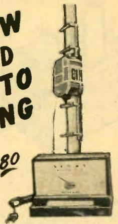
This rotator is packed with new features. Cartridge type power drive unit can be removed in seconds without dismantling antenna. Stop watch tuning accuracy within 1/2 degree anywhere in 360° rotation. Brakes to instant stop. Powerful balanced inline construction supports tremendous weight. Fingertip control with finely calibrated dial indicates precise antenna position at all times. Shpg. Wt. 12 lbs.
