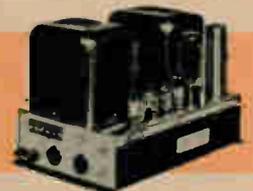
Superlative Amplification with 1M distortion at 1/2% and Harmonic Distortion at less than 1/4%. Input sensitivity 0.5 volt with gain control. Frequency Response ± 1 db between 15-50,000 cps. Hum and noise are -90 db. Amplifier outputs of 4, 8, 16 and 600 ohms (balanced). Tubes are 2-12AX7, 12-AU7, 12-BH7, 2-1614, 5 U4GA (Rectifier). Chrome and black finish. Dimensions 13 1/2" x 8" x 8". Power consumption 155 watts, 117/125v, 50/60 cycles AC. Shpg. wt., 34 lbs.
