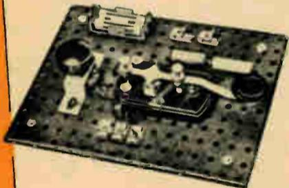
For those interested in mastering the international code, an audio tone oscillator is essential. The circuit of this transistorized feedback oscillator has the simplicity of the neon glow, the signal strength of service, vacuum tube, and requires only two penlite cells for weeks of service. It may be used for solo practice, or two may send and receive with the same unit. Kit comes complete with Tennantor, Telegraph Key, Resistor, Condensers, Masonite Board, etc., and Schematic Diagram.
