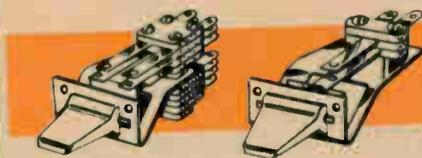
4PDT lever action switch has 4 sets of single-pole, double-throw contacts. Switch has three positions with positive and spring returns. Front panel mounting is especially suited for audio applications and intercoms. Mounts to panel with 2 screws, mounting centers 1" apart. Size 2 1/4" long behind panel, 1 3/16" wide, 1" high. Shpg. wt., 4 ozs. SW-68 4PDT Lever Switch Net .95
