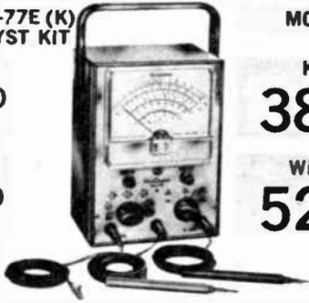
Easy-to-read 4 1/2" meter, 11 megohm input resistance. 28 ranges include 7 DC voltages: 0-1.5-5-15-50-150-500-1500, 7 AC rms voltages: 0-1.5-5-15-50-150-500-1500, ±5% of full scale accuracy; 7 peak-to-peak AC voltages: 0-4-14-40-140-400-1400-4000 volts; 7 overlapping ohms ranges from 0.2 ohms to 1000 megohms with center-scale values to 10, 100, 1000, 10K, 100K, 1 meg, and 10 megohms. Electronically protected against burnout. For 105-125 v., 50-60 Hz AC. With DC and AC/ohms probes and cables.
