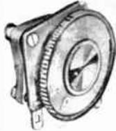
A new "Poly-Vari-Con" model for use in TRF broadcast-band and experimental receivers. Complete with good-looking clear plastic tuning dial with calibrations from 530 to 1600 kHz. Capacity variable from 10 to 365 pF. Knurled dial is 1 1/4" diam.; rotation is 180°. Dial is mounted to condenser shaft by 3/8" diam. chrome-plated threaded retainer. Imported.
