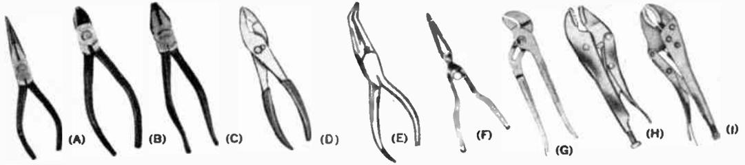
(A) **8 1/4" LONG NOSE PLIERS.** Durable drop forged steel pliers with hardened and tempered side cutting edges. Insulated handles for protection and comfort. Thin nose reaches into any space. Completely polished and lacquered finish to prevent rusting. Imported. Shpg. wt., 10 oz.
