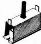
Exact replacement circuit breakers for television and industrial applications. Button must be pressed to reset. Tripping mechanism is temperature compensating for constant protection. Normal tripping time is 10 seconds or less. All values above 3.1 amps have special heavy-duty contacts to withstand heavy surge currents. Twist tab mounting lugs. Adapter for bushing mount listed below.
