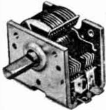
Lightweight—both the frame and plates are aluminum. Smooth ball bearing action over entire 180° rotation. Bake-lite stator insulation. Capacity of 11 plate R.F. section is 6.3 to 123.1 pF; 9 plate oscillator section is 5.7 to 78.2 pF. Effective range of trimmers is 15 pF. These add 2 pF to minimum capacity. Capacity increases in counter clockwise direction. Flatted shaft 1/4" diameter by 1/4" long. Frame size only 1 3/4"Dx1 1/2"Wx1 3/4"H. Shpg. wt., 5 oz.
