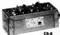
Utilizes a 6UBA mixer-oscillator, a 6ES8 cascode RF amplifier and specially designed transformers. High sensitivity. Noise figure—better than 4 db. IF rejection—over 100 db. Housed in 2 piece satin finished copper chassis. WILL NOT BECOME OBSOLETE, since the IF output can be easily changed to match any receiver. Size: 4 x 2½ x 5". Comes less power supply. Complete with tubes, crystal for 14-18 MHz IF output and instructions. Shpg. wt., 1 lb.
