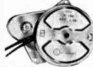
Self-starting synchronous motor with lifetime lubrication. Geared to 4 clockwise revolutions per hour. Will retain constant speed even under line voltage variations of 25%. Torque load 5 oz. in. maximum. Shaft ¼"x¼" dia. For 110-120 volt 60 Hz AC. Shpg. wt., 9 oz. 13 E 27246 Intermatic W-160 Net 3.30
