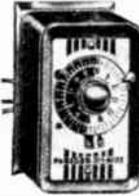
MODEL 101 compact time control ideal for window displays, night lights, yard lights, etc. Provides one on-off operation per day with minimum setting of two hours. Has manual trip lever. 24-hour dial is divided into 30 minute segments for easy, accurate setting. Fits over a U.S. standard single gang handy box. Size: 4½" Hx2¾" Wx3¼" D. Capacity: 15 amp. non-ind., 1800W, 1 HP. 12 amps., full load. For 120V., 60 Hz. UL and CSA Listed. 13 E 17510 Shpg. wt., 1½ lbs. Net 8.95
