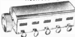
Five plunger operated tally registers in a single highly polished chromium plated case. Ideal for (1) laboratory use (2) time & motion studies (3) production control. Each 3-digit register counts up to 999. Easy-to-read numerals. Large knurled reset knob on side returns all 5 positions to zero simultaneously. Overall size: 5 1/4 x 1 7/8 x 1 1/4" D. Imported. Shpg. wt., 1 1/2 lbs. Net 9.95
