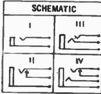
"LITTEL-PLUGS" PHONE PLUGS—Compact quality plugs. Fits standard 1/4" phone jacks except \* with .206 diam. sleeve and - with short sleeve for Revere recorders. In plastic handle or with brass nickel plated shells for shielding. Solder terminal has built-in cable clamp. Handle 1 1/4" long, 1/2" diam. Av. shpg. wt., 4 oz.
