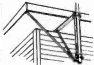
Permits mounting antenna to the underside of over-hanging eave. Can also be used as a sturdy self supporting flat roof mount. Heavy gauge steel and Hot-Dip galvanized for maximum corrosion resistance. One piece mounting of welded construction with a heavy gauge embossed steel diagonal support. Complete with installation hardware.
