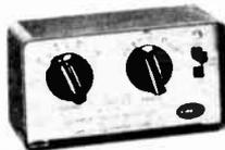
Model PCL improves receiver reception. Covers 6 through 160 meter amateur bands continuously. Uses 2 6DS4 Nuvistors in a cascode circuit for greater receiver gain and extremely low noise figure of 1.8 to 3.5 db. Also improves image and spurious rejection. Controls: 4-position range switch (1.8 to 54 MHz); Antenna Tuning Control, and 3 position switch for On, off and standby. Built-in 117 VAC power supply. Size: 5½ x 3¾ x 3"D.
