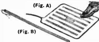
**Tapeswitch Flexible Switch Mats (Fig. A).** Less than 5 lbs. pressure activates these mats. Although rated and tested at 1 amp., 117VAC for floor switching, 24-volts or less is recommended. Only 3/32" thick; water-resistant durable covering. Shpg. wt.: 17 x 23" mat, 1 lb.; 6 x 23" mat, 6 oz. 17 x 23" Mat with 6' Cord.
