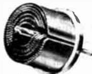
Fits any electric drill or drill press. Cylindrical saw blades cut holes from 1" to  $2\frac{1}{2}$ " in diameter in any stock up to 2". Hole sizes are 1",  $1\frac{1}{4}$ ",  $1\frac{1}{2}$ ",  $1\frac{3}{4}$ ", 2",  $2\frac{1}{4}$ ",  $2\frac{1}{2}$ ". Cut wood, plastic, metal, sheetrock, wall-board, masonite, formica, etc. Has guide bit and automatic slug ejector. Imported.
