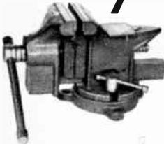
This favorite machinist vise swivels full 280° Width of Jaw: 4". Geared bolt and base plate give positive lock against slippage. Removable hardened pipe jaws open to 4¾"; plated screw bar. Steel handle balls forged from handle stock. Precision machined malleable iron castings. Self-lubricating graphite bronze bearing. Imported. Shpg. wt., 16 lbs.
