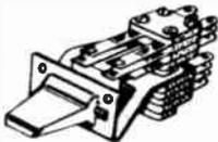
4PDT Audio Lever Switch: Has 2 dual sets of single pole, double throw contacts. One set is momentary contact-spring return, (press-to-talk). In the reverse position of the lever (dictate), the second set of contacts remain in the positive position until released. Panel mounting, mtg. centers 1" apart. Size 2 1/4" long behind panel. 1 1/2" W x 1" H. Imported. Shpg. wt., 3 oz. 99 E 61542 Net ea. .99
