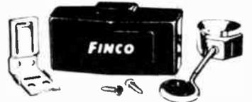
MODEL 3007. Eliminates interference from citizen band, amateur operators, electric motors, aircraft, fluorescent lamps and auto ignition. Provides up to 40 db attenuation of all interfering signals outside the FM band. Less than 1 db insertion loss in 88 to 108 MHz band. Recommended to be mounted at FM radio set for maximum effectiveness but may be mounted anywhere in line for less serious applications. 18 E 30165 Shpg. wt., 8 oz. Net 4.38
