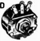
Dust-proof phenolic case 1 1/2" diameter. Insulated contact arm type 900 V. AC insulation. All have linear taper. Knurled screwdriver slotted stub shaft with 3/8" standard bushing. With nut.
