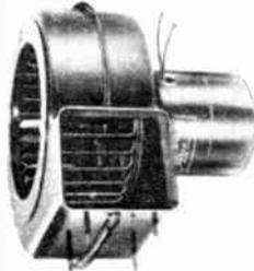
Heavy Duty centrifugal blower usable in many applications—air distribution in confined areas, exhaust fumes and gas, etc. Suitable for ventilation equipment in home, marine, and commercial use. Provides efficient quiet operation. 10" A.C. leads for 115VAC. 60 Hz .64 Amp. Shpg. wt., 8 lbs.
