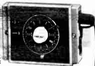
Smartly styled wall timer with finger-tip control. Installs easily in standard, single outlet wall box. Automatically controls air conditioners, lamps, radios, coffee makers, and any other plug-in appliance. Resets automatically. 1 timed AC outlet and 1 AC outlet completely independent of timer. May also be used manually. Minimum "ON" time: 15 min. Maximum "OFF" time: 23 hr. 45 min. Capacity: 15 amps, 125 volts, 60 Hz. Compact, only 1¼" above wall, Pearl white housing.
