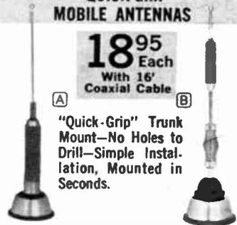
(A) Model M175. Base Loaded Antenna with attractive gray jacket and chrome end fittings. Stainless steel whip. Whip adapter provides 1 1/4" adjustment for extra fine tuning. "Quick-Grip" mount. Solderless lead connection with PL-259 at set end of 16 foot coaxial cable. Shpg. wt., 1 lb.
