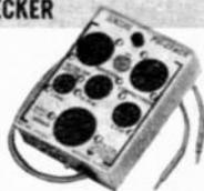
Check continuity of all tube filaments including the new Compactrons, Novars, 10-pins, Nuvistors and the new Decals. Test leads for CRT filament checking. Also doubles as neon voltage indicator. 4 x 3 x 1". Shpg. wt., 1 lb.
