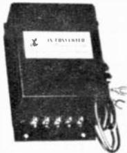
Permits you to match voltage and polarity from any 6 or 12 volt DC power source to your citizens band equipment. Converts 6 volts DC to 18, 12 volts DC to 24. Inverts polarity from positive to negative to positive. Select any combination of connections in seconds by merely changing one jumper cable. Size: 5 3/4" L x 2 1/2" H x 3 3/4" W. Shpg. wt., 2 1/4 lbs. **42 E 39190** .....Net 22.95
