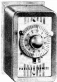
MODEL 101 compact time control ideal for window displays, night lights, yard lights, etc. Provides one on-off operation per day with minimum setting of two hours. Timer will repeat this on-off schedule once every 24 hours. Has manual trip lever. 24-hour dial is divided into 30 minute segments for easy, accurate setting. Fits over a U.S. standard single gang handy box. Size: 4½H x 2¾W x 3¼"D. Capacity: 15 amp. non-ind., 1800W. 1 HP, 12 amps., full load. For 120V., 60 Hz. UL and CSA Listed.
