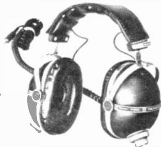
2-way dynamic headphone for extended frequency response. Each earpiece contains a separate woofer and tweeter, employing a polyester film diaphragm for excellent transient response. The SE-505 also contains independent volume and tone controls for each channel. Adjustable sliding foam filled headband. Matches impedance 4 to 16 ohms. Response: 20-20,000 Hz. Imported. Shpg. wt., 3 lbs.
