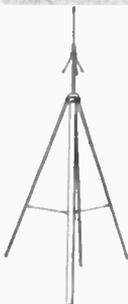
Provides 5 db gain over a flat ground plane. 100-mph-plus wind survival. Waterproof coax feedpoint. Handles in excess of 2500 watts. Best signal lobes at the horizon. No up-angle of radiation. Diecast aluminum and seamless aircraft tubing construction. Simple to assemble and install. Static cap at radiator midpoint for best S/N ratio. Can be mounted on 1" threaded pipe or 1 1/4" steel mast. Overall height 18 ft. Parcel Post Shippable. Shpg. wt., 5 1/2 lbs.
