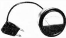
Type 5406-LT. Sturdy, pocket-sized tester has a range of 0-150 volts AC/DC. Plug into any wall outlet and read the voltage. Then plug in the appliance(s) and note the new reading. Find (and demonstrate) voltage drop or inadequate wiring as a source of service problems. Shpg. wt., 6 oz.
