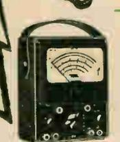
Brand new laboratory-precision 20,000 ohms/volt multimeter featuring greatest ranges, accuracy and ruggedness of construction. 31 different full scale ranges. DC/AC Voltage: 0-2.5, 10, 50, 250, 1000, 5000. DC Current: 0-100 ua, 10 ma, 100 ma, 500 ma, 10 amp. Ohms: 0-2000, 200K, 20 megs. 5 DB Ranges: -12 to +45. Large 4 1/2" 60 ua meter movement. Hand-calibrated and tested rectifier. High-impact bakelite case. 6 1/4" x 3 1/4" x 3". Shpg. wt. 3 lbs.
