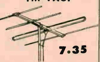
A broad banded 4 element Yagi for high gain on FM band, 88 to 108 MC. All aluminum construction with square boom; special "Lock-Tite-No-Tilt" saddle bracket for permanent horizontal alignment. Reinforced elements are pre-assembled with snap-out brackets. Impedance step-up design for maximum energy transfer. Shpg. wt., 5 lbs. FINCO FM-3 ..... Net 7.35
