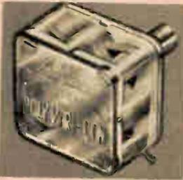
Two-gang midget variable for top performance in transistor superhet circuits. Capacitance of antenna section, 10 to 208 mmf, and 10 to 100 mmf on the cut oscillator section. Self-contained trimmers. Tunes through 180°. Enclosed in transparent plastic case. Offers unlimited possibilities to the experimenter.
