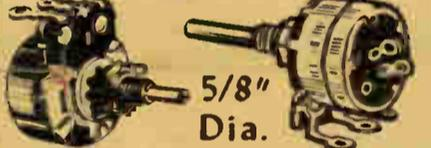
For Transistor and Sub-Miniature Circuits Versatile carbon controls for audio, tone and similar applications; specially designed for Transistor and Sub-miniature circuits. Only 5/8" diameter. Shaft 1" long 1/8" diameter. Shaft easily cut to desired length, includes nut and lock washer. Shpg. wt. 2 oz.
