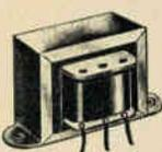
Power Output Transformer for 6L6, 25L6-GT, 35L6GT, 117N7G-T, etc. To 500 Ohms or 6 to 8 Ohm voice coil. (Separate windings.) Open type mounting—3 3/4" centers. With leads. Shpg. wt. 3 lbs.
