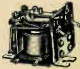
Double pole relay, with one set of SPST contacts normally open, and one set of contacts normally closed, contacts of  $\frac{1}{16}$ " fine silver, rated at 550 watts non-inductive load at 60 Cycles. Coil operates on 14 to 32 volts, with DC resistance of 27.5 Ohms. Overall size, 2"x2 $\frac{1}{4}$ "x1 $\frac{1}{8}$ ", with mtg. bracket.
