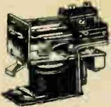
Three pole relay, with two sets of SPST contacts normally open, and one double make contact, normally open, all contacts of  $\frac{1}{16}$ " fine silver, rated at 50 watts non-inductive load at 60 cycles. Coil operates on 20 to 29 volts AC, with DC resistance of 30 ohms. Overall size, 2 $\frac{1}{2}$ "x2"x1 $\frac{1}{2}$ ".
